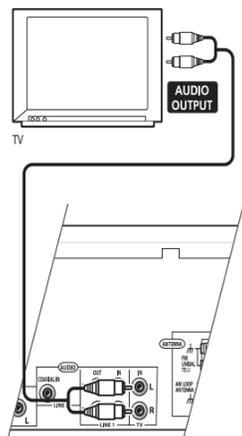
Connect a stereo audio cable (not supplied) from the audio outputs of your TV to the **TV IN** jacks on this system.
