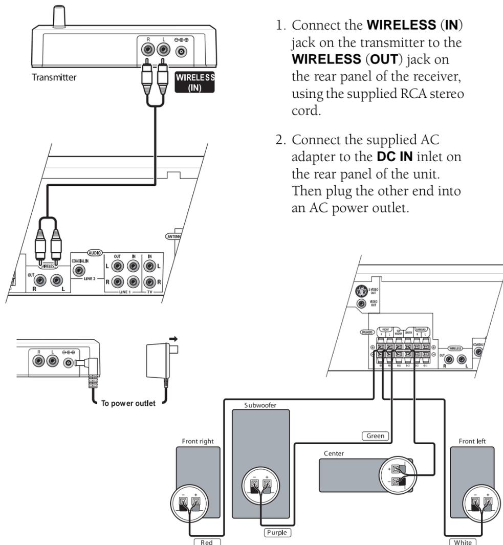
1. Connect the **WIRELESS (IN)** jack on the transmitter to the **WIRELESS (OUT)** jack on the rear panel of the receiver, using the supplied RCA stereo cord.
