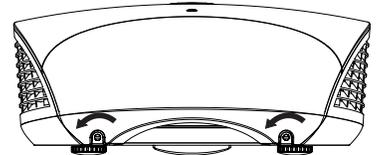
Then, remove the rear compartment cover by tilting it upward.
