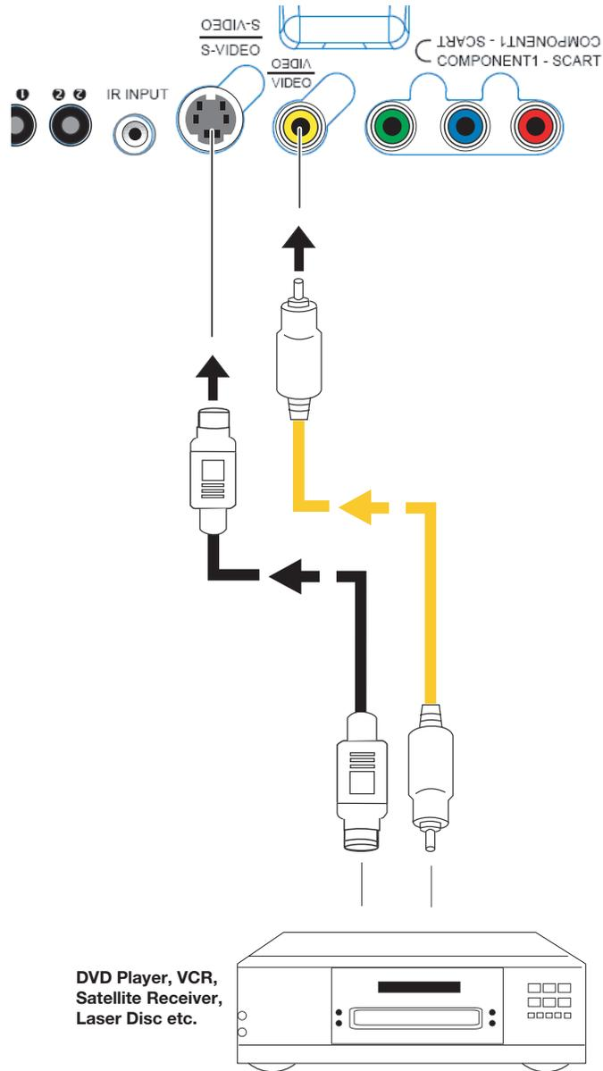
**Figure 3-10. Composite and S-Video Connections**
