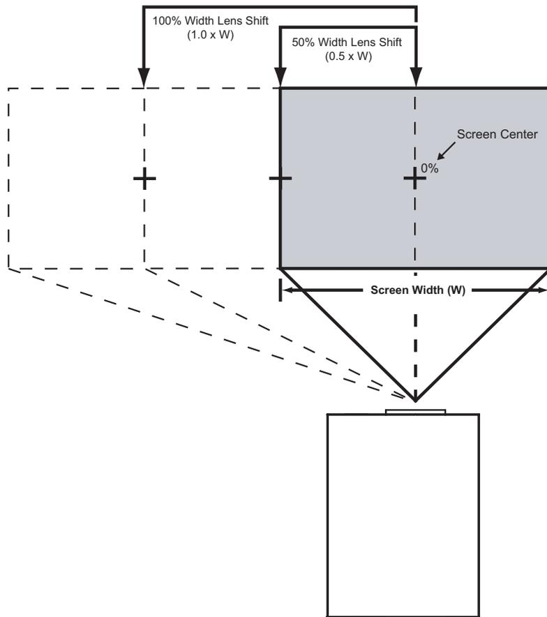
**Note:** This is a general example of lens shift. Lenses vary in their shift capabilities. **No particular lens or projector is used in this example.**
