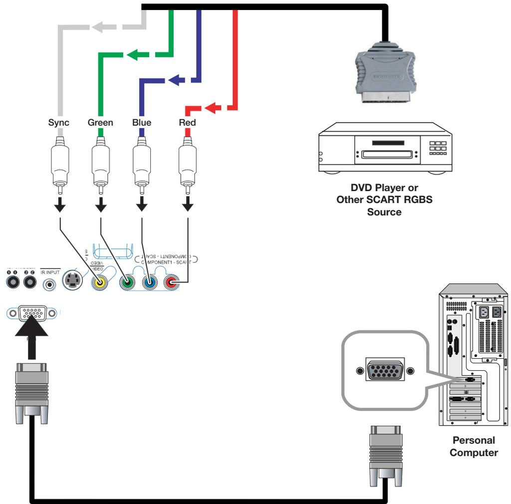
Figure 3-8. RGB Connections
