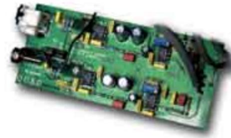
The standard QC-twenty-four is line level only. There is an option of a solid-state phono stage which can be added when new, or at a later stage.
