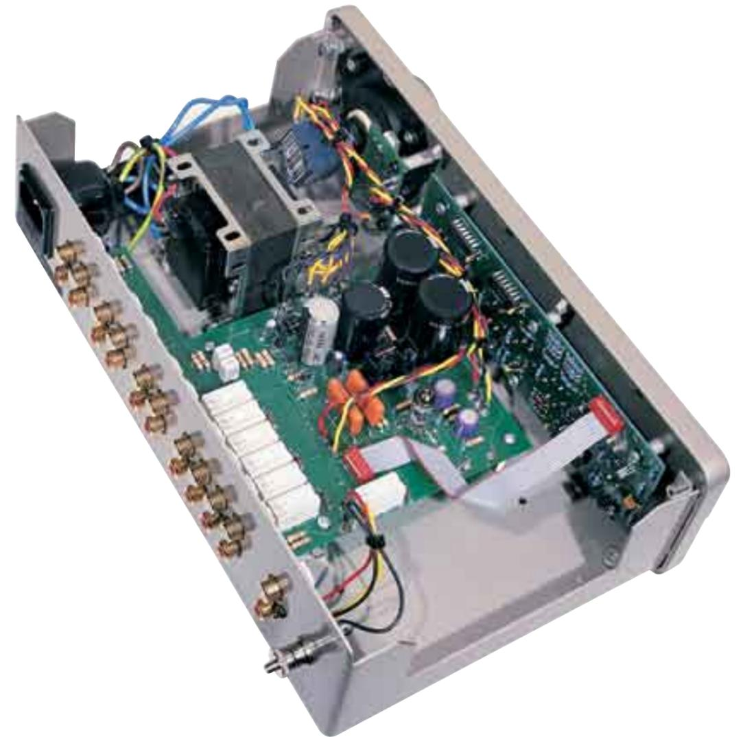
A completely new design, the QC-twenty-four pre amplifier is both neutral and detailed. Using a military specification 6111 valve, which is so reliable, it's hard-wired to the circuit board.
