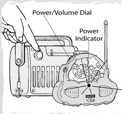
Place transmitter in room in which you intend to use it. Rotate transmitter power/volume dial to turn power on. Turn on a radio.
