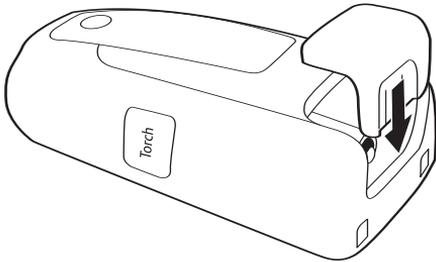
3. Slot the Parent unit into the charger, the red charging light comes on. Charge the batteries for 16 hours before switching on the Parent unit.
