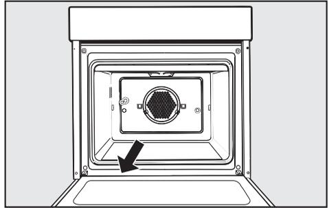
The silver data plate is located along the front side of the oven (door open).
