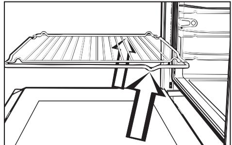
Once inserted into the oven these pieces can only be removed by raising the piece upwards and then pulling it out.
