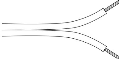
3. Press the speaker's black negative (-) terminal tab and insert one of the bare wire ends into the opening. Then release the tab.
