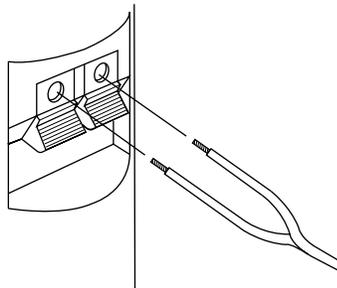
4. Press the speaker's red positive (+) terminal tab and insert the other bare wire end into the opening. Then release the tab.
