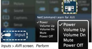
Inputs > AVR screen. Perform NetCommand IR "learning" for A/V receiver power and volume keys.
