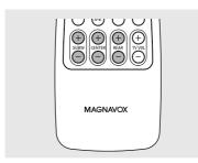
Press the respective buttons on the remote (REAR + -, CENTER + - and SUBW + -) to adjust the output level between -15dB ~ 10dB.
