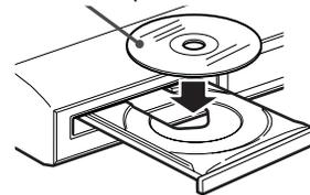
When placing an 8 cm disc
