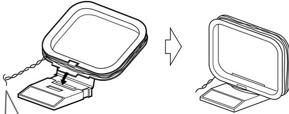
If the antenna cord is covered with the insulation coat, twist and pull the insulation coat off and remove.
