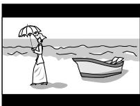
Select this option for playback on a TV with a height/width ratio of 4:3. The image will be displayed with a black bar at the top and bottom of the screen. The left and right edges of the image are preserved.
