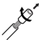
Twist and remove the insulation at the end of each speaker cord.
