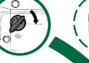
Set engine switch to "ON" ("RUN").
