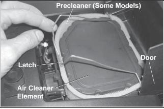
Figure 12. Unhooking Latch (Courage).
