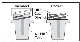
Figure 6. Thread-on Oil Fill Cap/Dipstick.
