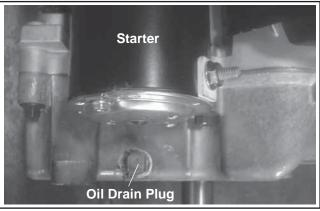
Figure 8. Oil Drain Plug.
