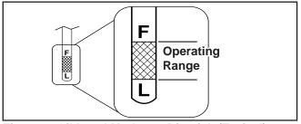
Figure 7. Oil Level Marks on Dipstick (Typical).
