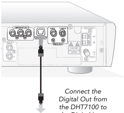
Connect the Digital Out from the DHT7100 to the Digital In on your A/V receiver.
