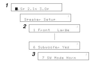
Select "Large" or "Small" not according to the actual size of the speaker but according to the speaker's capacity for playing low frequency (bass sound below the frequency set for the Crossover Frequency) signals. If you do not know, try comparing the sound at both settings (setting the volume to a level low enough so as not to damage the speakers) to determine the proper setting.
