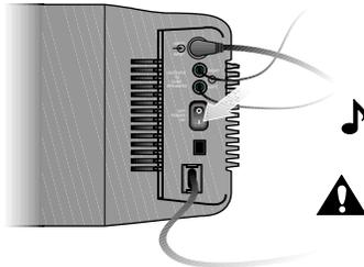
1. Plug the Acoustimass® module power cord into an AC power (mains) outlet.
