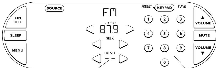
Press and hold here to store a preset or, to quick-store a preset, press and hold any button 1 through 9.
