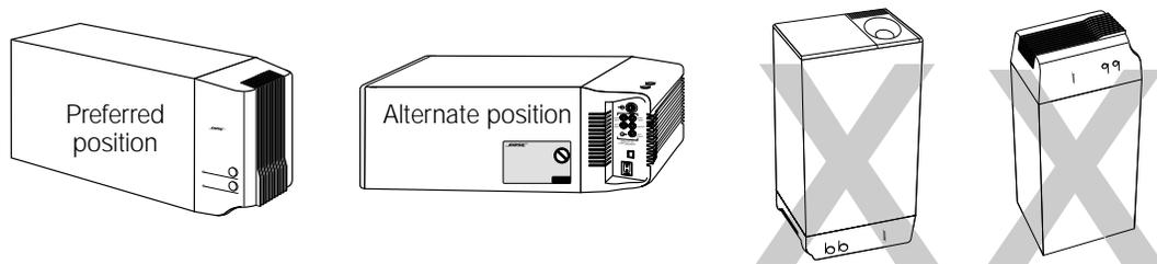
5. Once you have selected a position for the module, place the four self-adhesive rubber feet near the corners of the bottom surface. The rubber feet provide increased stability and protection from scratches.
