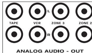
**For ZONE2, ZONE3, and RECORD to have any output, the source components being used there must be connected to the AVM 50 with the same type of connection. For example, if you're using HDMI video output for MAIN, to use ZONE2, the source components must be connected to the AVM 50's inputs (in addition to HDMI) with analog L/R for audio, plus Component video, S-Video, or Composite video – whichever type the display in ZONE2 uses.**
