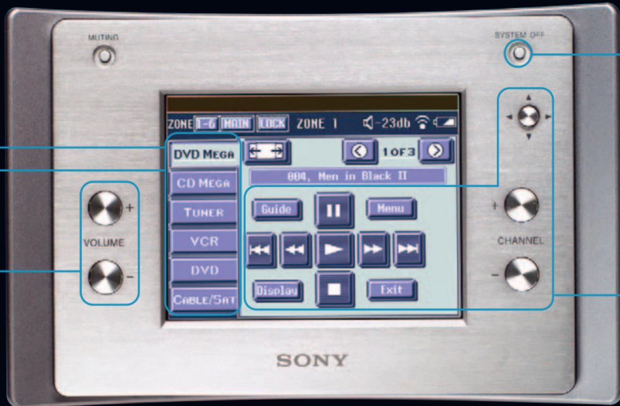
**WHEN YOU'RE DONE** – press the **SYSTEM OFF** button, then hit the **ALL ZONE OFF** button on the LCD screen. The entire system will shut down.
