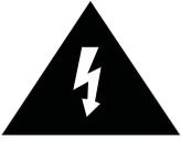
The lightning flash with arrowhead symbol, within an equilateral triangle is intended to alert the user to the presence of un-insulated “dangerous voltage” within the products enclosure that may be of sufficient magnitude to constitute a risk of electric shock to the persons.
