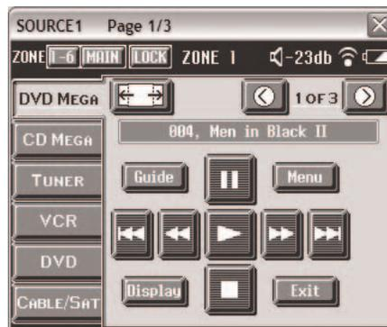
2. For most sources, the RF Remote Commander unit offers several "pages" of virtual buttons. On this screen for example, "1 of 3" indicates three pages of buttons. Use the **PAGE BACK** and **PAGE FORWARD** virtual buttons move between pages.
