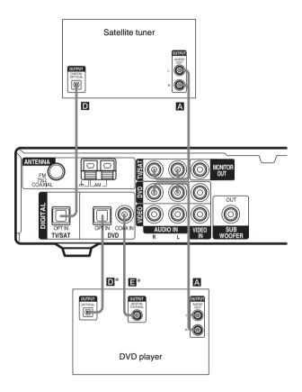
\* Connect to either the COAX IN or OPT IN jack. We recommend making connections to the COAX IN jack.
