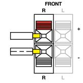
8. Place the other end of the plain wire into the red (+) terminal on the back of the speaker that you placed to the right of your TV set. Place the other end of the black-striped wire into the black ( - ) terminal of the same speaker.
