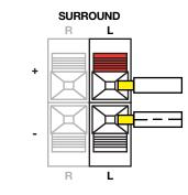
**12.** Place the other end of the plain wire into the red (+) terminal on the back of the surround speaker that you placed on the left side of your room. Place the other end of the black-striped wire into the black ( - ) terminal on the back of the same surround speaker.
