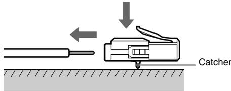
With the catcher facing down, press and hold the plug down against a flat surface and remove the cords from plug.
