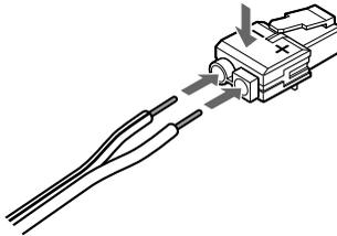
While pressing the plug down against a flat surface, insert the new speaker cords. Note that the cord marked with a line should be attached to the minus (-) side of the plug.
