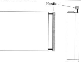
Handle used in disk module insertion.
