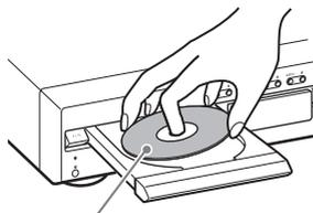
When you play an 8 cm disc, place it on the inner circle of the tray. Be careful that the disc is not skewed on the inner circle of the tray.
