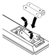
Detach the battery cover on the rear of the remote control, and insert two R03 (size AAA) batteries with **+** and **-** aligned correctly.
