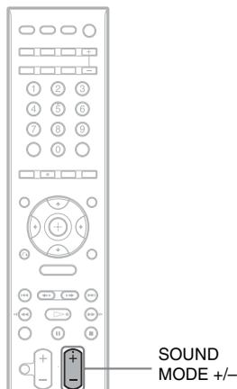
**Press SOUND MODE +/- repeatedly during playback until the desired mode appears in the front panel display.**
