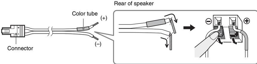
When connecting to the unit, insert the connector until it clicks.
