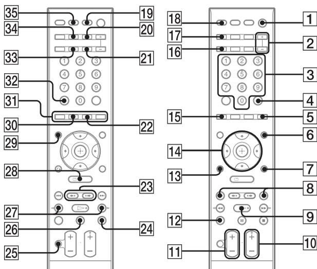
\* The ENTER button has the same function as the ⊕ button. When you operate the TV, the ENTER button is used for selecting a channel, and the ⊕ button is used for selecting menu items (page 83).
