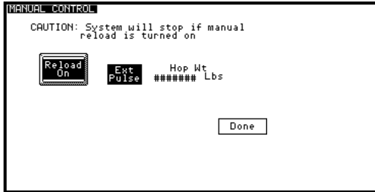
Figure 34: Typical Manual Control Operator Screen
