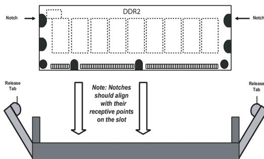
**To Remove:** Use your thumbs to gently push each release tab outward to free the DIMM from the slot.
