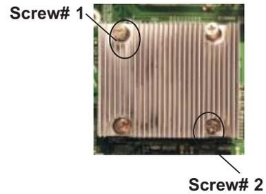
2. Hold the heatsink and gently wriggle the heatsink to loosen it from the processor. (Do not use excessive force when wriggling the heatsink!!)
