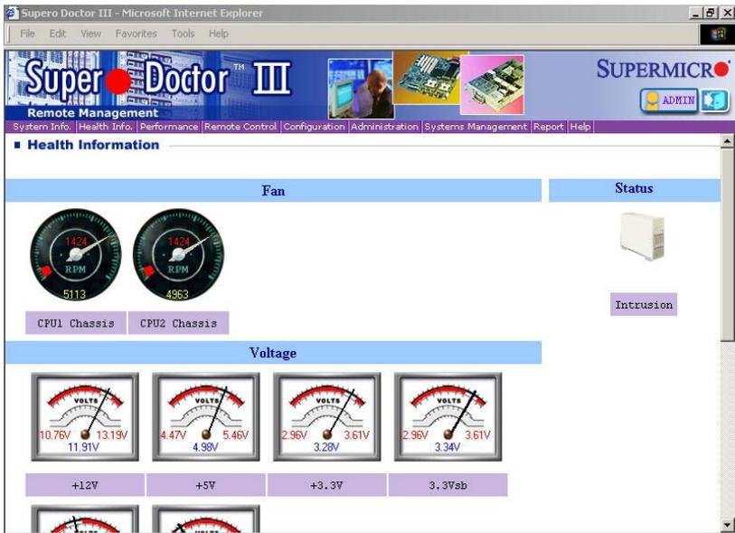
Figure B-3. Supero Doctor III: Remote Control Display
