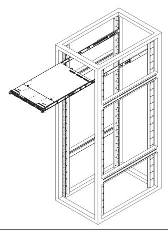
Figure 2-3. Installing the Server into a Rack
