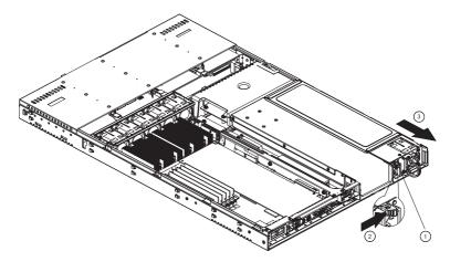
Figure 6-5. Removing/Replacing the Power Supply
