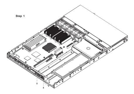
Figure 6-6. Reconfiguring the Power Supply
