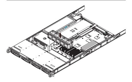
Figure 6-2. Removing the Fan Housing
