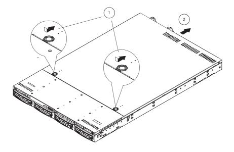
Figure 2-5. Accessing the Inside of the System
