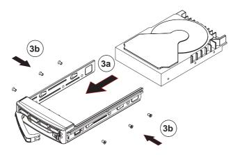
Figure 6-3. Mounting a SCSI Drive in a Carrier
