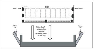
Figure 5-5a. Side View of DIMM Installation into Slot
