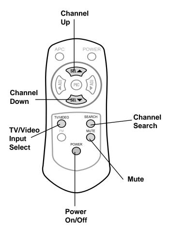
NOTE: Some buttons on the AC3105 remote control do not operate with the AC3105 - they are for other applications using optional equipment. All operating buttons are highlighted in the diagram above.
