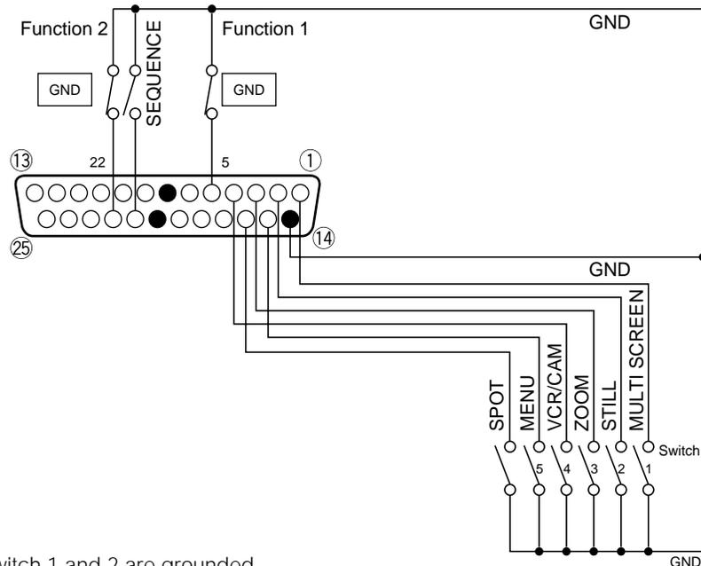
**Note:** Make sure that Function switch 1 and 2 are grounded.
