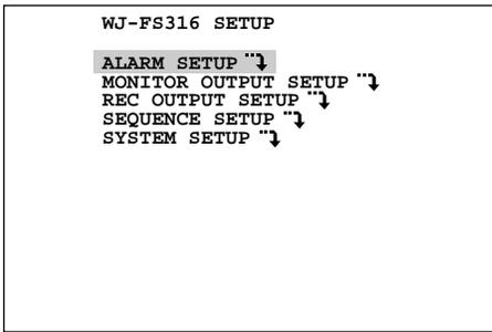
Move the cursor to ALARM SETUP on the SETUP menu, then press the **SET** button. The ALARM SETUP menu appears on the monitor screen as shown below.
