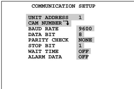
Move the cursor to COM. SETUP, and then press the **SET** button. The COMMUNICATION SETUP menu appears on the monitor.
