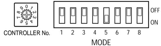
1. Rotate the CONTROLLER NO. switch to set the controller number.
