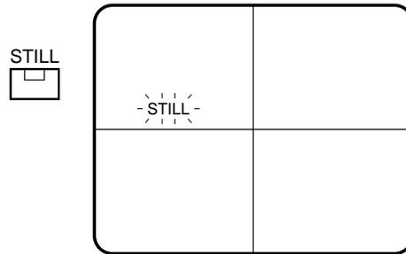
3. Press the **CAMERA SELECT** buttons 1-16 (9) to freeze the displayed picture. **STILL** blinks in the display.
