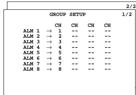
1. Move the cursor on GROUP in the DYNAMIC REC line and press the **SET** button to open the GROUP SETUP menu shown above.
