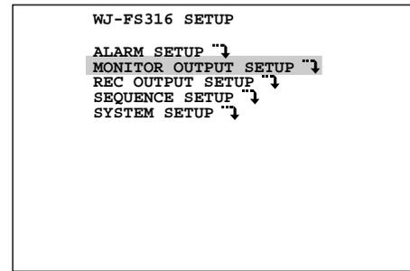
Move the cursor to MONITOR OUTPUT SETUP on the SETUP menu, then press the **SET** button. The MONITOR OUTPUT SETUP menu appears on the monitor screen as shown below.
