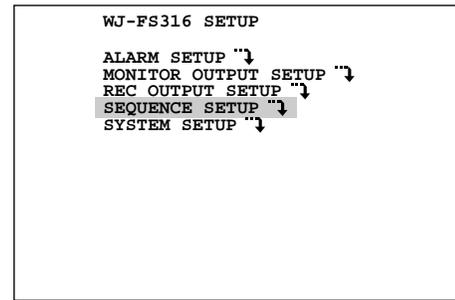
Move the cursor to SEQUENCE SETUP on the SETUP menu, then press the **SET** button. The SEQUENCE SETUP menu appears on the monitor screen as shown below.
