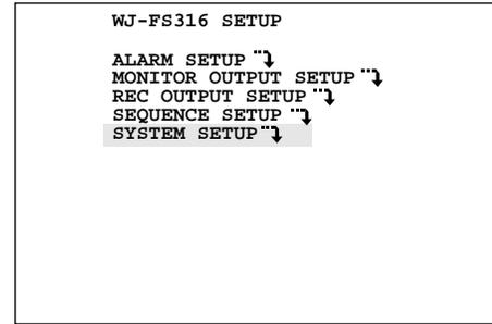
Move the cursor to SYSTEM SETUP on the SETUP menu, then press the **SET** button. The SYSTEM SETUP 1/2 menu appears on the monitor screen as shown below.
