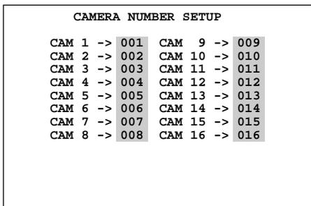
2. Move the cursor to the desired CAM line, and then select a camera number by pressing the **+** or **-** button.
