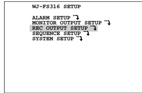
Move the cursor to REC OUTPUT SETUP on the SETUP menu, then press the **SET** button. The REC OUTPUT SETUP menu appears on the monitor screen as shown below.
