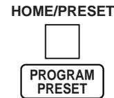
2. Select a preset position number using the numeric buttons, then press the **HOME/PRESET** button to move the camera to the position.
