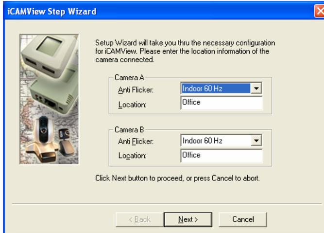
4. Enter the necessary camera configurations. Choose the appropriate frequency (Indoor 60 Hz, Indoor 50 Hz or Outdoor) to prevent flickering on the video feed. Enter a name for the camera in the “Location” box to easily identify it.
