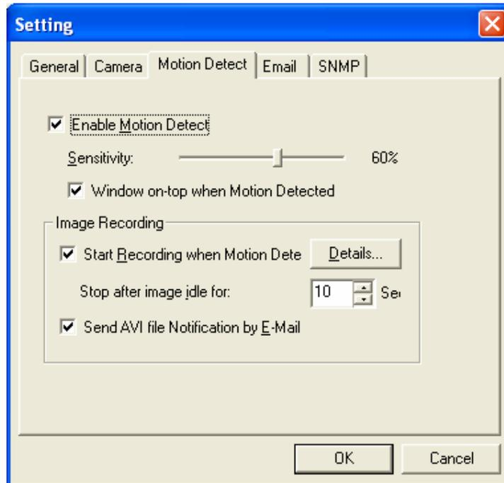
**Enable Motion Detect:** Click the checkbox to enable Motion Detection.
