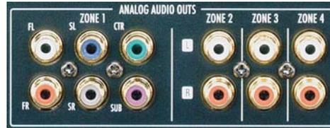
Figure 4 – Analog Audio Outputs
