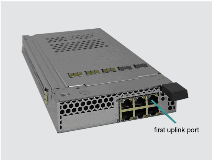
Figure 14: First uplink port of an IBP module
