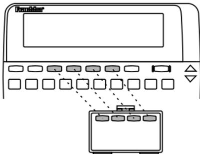
*Remember, when you have selected and are using a BOOKMAN cartridge, the color keys function as labelled on that cartridge, not as on the keyboard.*
