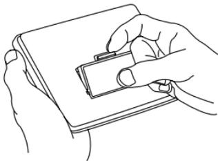
4. **Press the cartridge down until it snaps into place.**
