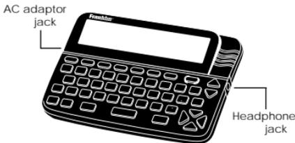
**AC adaptor jack:** Some BOOKMAN models are equipped with a standard 3.5 mm jack for use with a 9-volt, 200-300 milliamp AC/DC adaptor.
