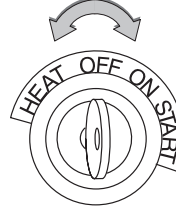
Typical starter switch
