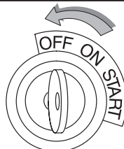
Typical starter switch
