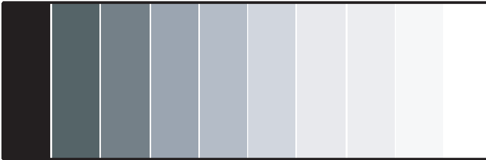
Figure 4-3. Typical Gray Bar Pattern for Adjusting Contrast
