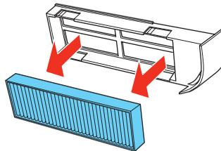
5. Gently tap both sides of the air filter against a hard surface four or five times to remove loose dust from the air filter.
