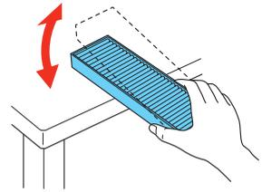
6. Use a small vacuum cleaner that is designed for computers and other office equipment to remove any remaining dust from the surface of the filter. If you don't have one, gently clean the filter using a very soft brush (such as a clean artist's paintbrush).
