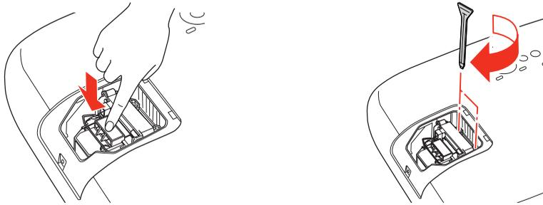
9. Replace the lamp cover. (The projector won't work if the lamp cover is open or loose.)
