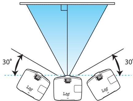
If one side of the image is taller than the other, make sure the projector is parallel to the screen. If necessary, adjust the front feet so that the projector is horizontal.
