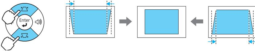
In addition to the horizontal keystone slider, you can use the volume buttons on the projector to adjust images that are wider on the left or right side.
