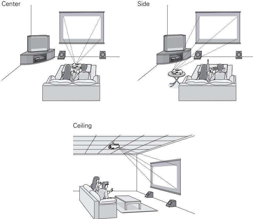
Keep the projector level and place it at a height where its lens is centered between the top and bottom of the screen. If this isn't possible, use the horizontal keystone slider and vertical keystone buttons to adjust the image (see page 24).
