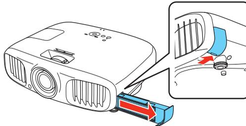
4. Remove the air filter as shown.
