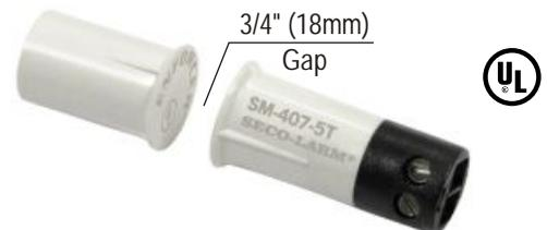
*These SECO-LARM contacts incorporate **Gold-Plated Terminals** to help increase the life of the contact. In addition, most SECO-LARM magnetic contacts incorporate reed switches with a superior breakdown voltage and a deactivated rhodium plating to eliminate absorption of organic impurities, polymer growth during operation, and the possibility of contact freezing, especially at the lower voltage levels normally used in security systems. SECO-LARM offers the most reliable contacts.*
