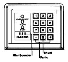
Faceplate of Digit-Key keypad lifts up to reveal convenient reference index of zones protected.
