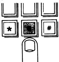
To arm with zone(s) shunted, first check the green STATUS lamp to make sure that no perimeter zone is in "trouble". Then press the SHUNT button, labeled "S", and enter your code. The yellow SHUNT light and the red ARMED/MEMORY light will come on. The green light will be out. The SHUNT light will go out when you disarm the Control Center.
