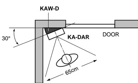
Connect wires, attach back frame to KAW-D and remount KA-DAR.
