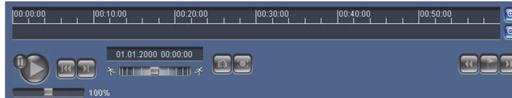
A time bar below the video image allows quick orientation. The time interval associated with the sequence is displayed in the bar in gray. A green arrow above the bar indicates the position of the image currently being played back within the sequence.
