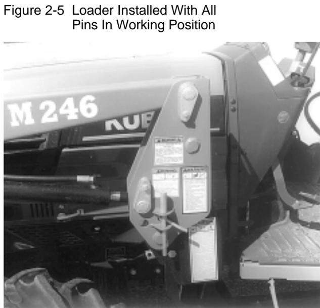
F. Extend lift cylinders slowly making sure loader is seated completely in mounting bracket top and bottom receivers. Retract bucket cylinder until bucket is approximately 1/2" off ground.
