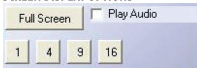
**Full Screen** – Opens current viewing screen to full screen mode. To exit, right click the mouse. **(Note: There are no playback controls on full screen)**
