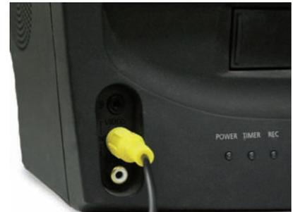
1. Connect a BNC to RCA connector to the MONITOR OUT connection on the back of the DVR.
