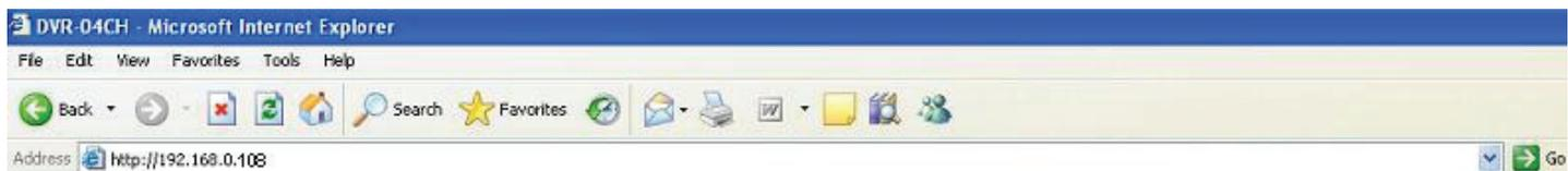
If the computer and the DVR are connected to the same router you can use the internal IP address to view the DVR. If the computer is not connected to the same router and is at a remote location you will need to use the external IP address for the DVR to view the DVR from that computer.
