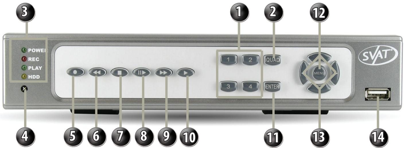
1. Channel Display buttons – Displays each corresponding camera channel in full screen when selected
