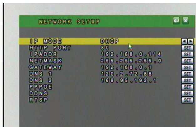
**If your router does not support DHCP, contact your network administrator to supply you with the proper IP information. If the DVR needs to store PPPoE (DSL/ADSL) settings contact your ISP (Internet Service Provider) for the proper IP address settings.**
