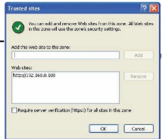
*The IP address used in the example above is for internal network viewing. If you are trying to access the DVR from a remote location you will add the "External IP Address" to the trusted sites list. See Finding your External IP Address.*
