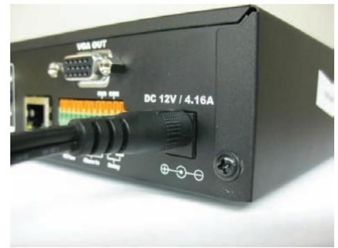
1. Insert the power cord into the power supply.
