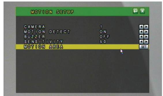
**Note:** Every time motion is detected an icon will appear, and the camera name from which motion is detected will change from white, to yellow.
