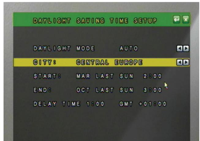
**Manual:** Manually set the start and end date and time for daylight savings in your area. The delay time will be the time difference during the daylight savings month. Ex. If the time changes 1 hour behind then the delay will be set to 1 hour.
