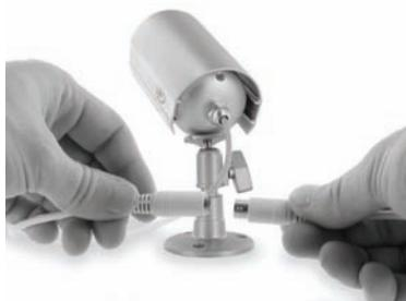
2. Plug the included four port power supply into the camera power adapter then into the red power jack located on the 60 ft video/power wire.
