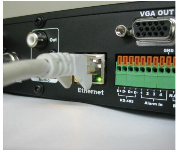
**Note:** *If you look at the router there should be a green "link" light indicating that the DVR is properly connected to the port that it was plugged into. There will also be an amber and green "link" light to the right of the Ethernet connection on the back of the DVR to indicate a proper connection to the router. If both "link" lights are illuminated, the DVR is properly connected to the router and you can proceed with the next step.*
