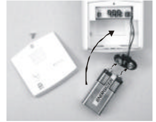
Insert 9V alkaline battery to the sensor
