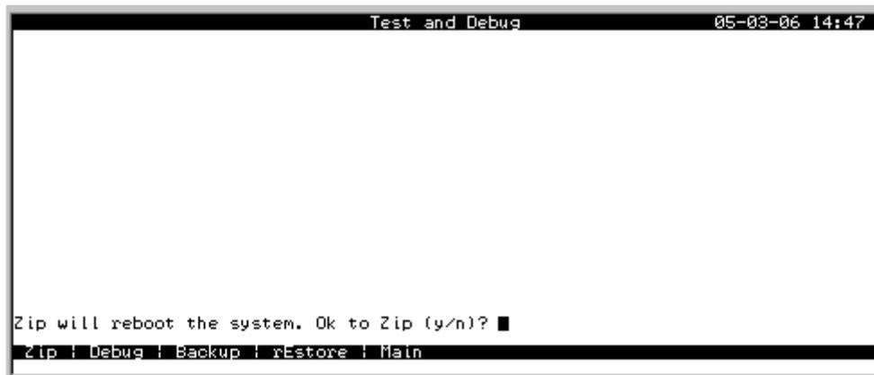
**Figure 3-9.**Cold-Start NVRAM "Zip"Test and Debug Screen.
