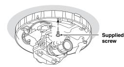
Make sure that the camera unit and base plate fit perfectly.
